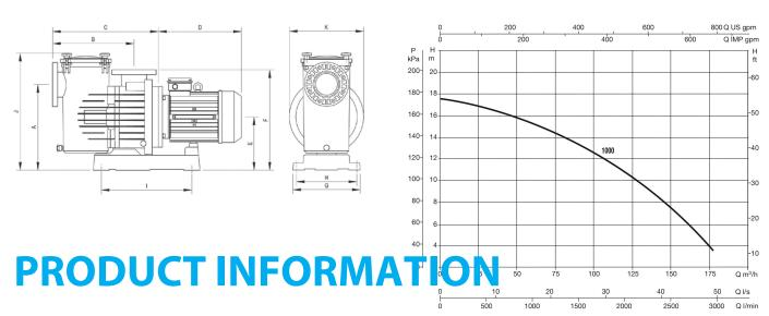
High performance self-priming centrifugal electric pumps with built-in high capacity prefilter. 2 or 4 pole motor completely isolated from the water. Extremely quiet and highly reliable, developed for water circulation and filtration in large swimming pool filtration systems. Thanks to the AISI 316 mechanical seal, they are also suitable for specific applications for the circulation of sea water.
